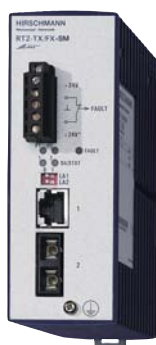
100 BaseTX to 100 BaseFX, SC, Single mode
