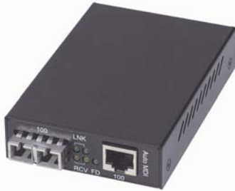
100 BaseTX to 100 BaseFX, SC, Multimode
