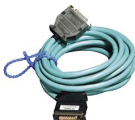
Connection cable Multiplexer – PLC TTY
