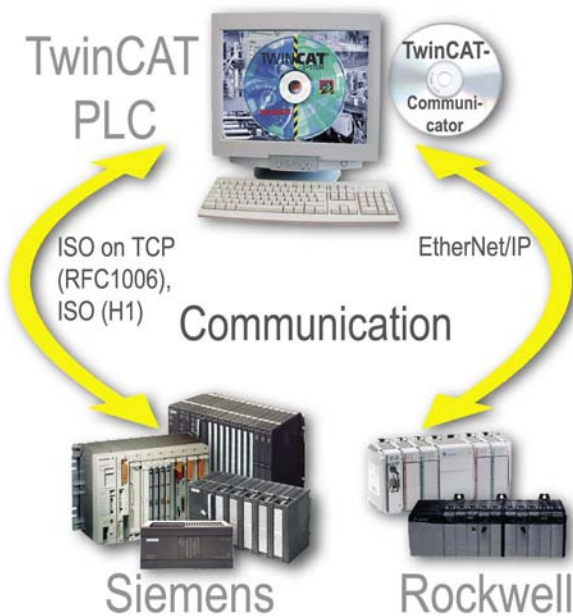
Communication of the TwinCAT PLC with Siemens and Rockwell
