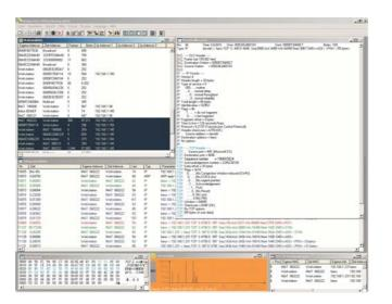
Using these displays you can observe the network communication, and find the source of any disturbances or faulty frames.
