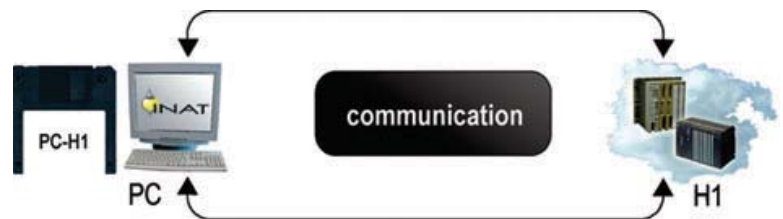
Access to S7 and S5 PLCs with PC H1
